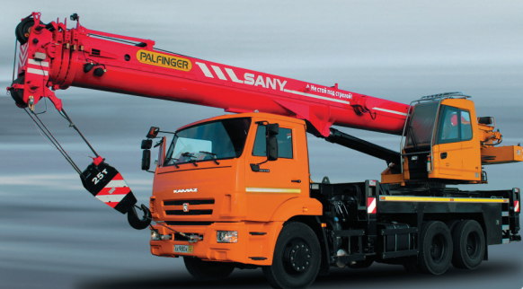
32 TONS TRUCK CRANE BOOM 10.2-32 m
