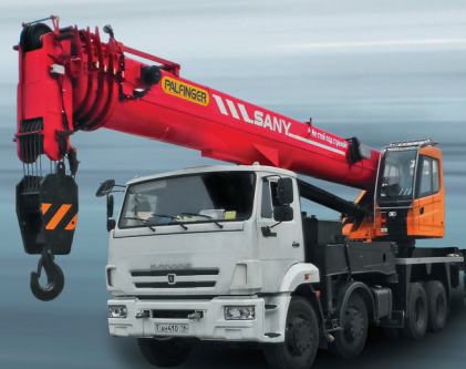
40 TONS TRUCK CRANE BOOM 10.5-49.51 m
